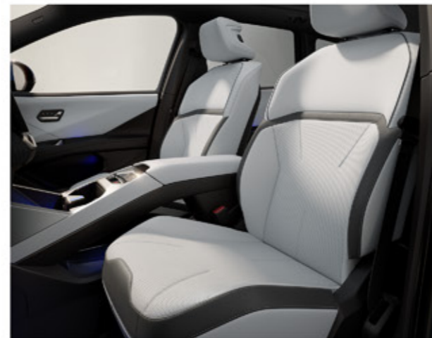
Multifunction seats for driver and front passenger , can be adjusted electrically, include memory function, 7 massage programs for the front seats and lumbar support.
