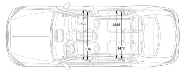
All figures in millimetres. The pictured dimensions are mean values. They are valid for vehicles with standard equipment and in unladen condition.
