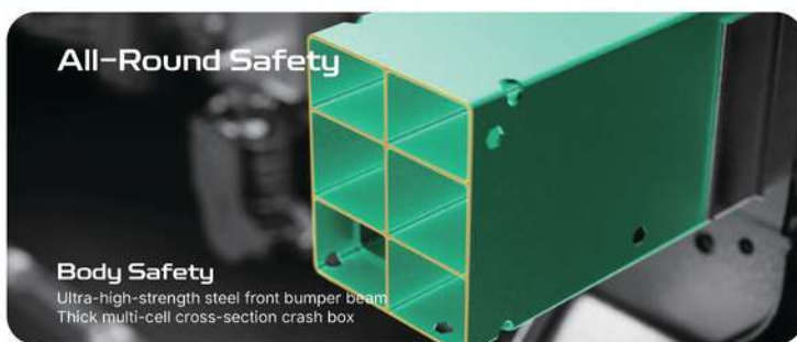
Three-Tier Stepped Chassis Safety Design
